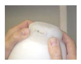
the flexible inner socket from the laminated frame. (To keep the flexible inner socket from being locked into the frame). Also fill the threaded hole in the tab with putty, in case of leakage while laminating.
